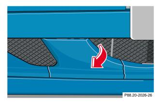
The rear towing eye is located at the right, below the bumper. The front towing eye is located on the passenger side behind a cover in the bumper panel.
